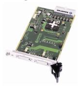
The CP332 provides two DVI-I connectors on the front panel enabling the user to connect up to two analog or digital monitors to the CP332.
