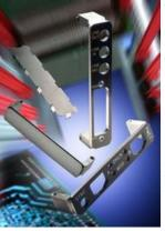
The bezels are available either in extruded aluminum with 240 grit graining and a clear alodine finish, or in die-cast zinc with a zinc finish. Both types are supported by flexible silkscreen and CNC machining to produce custom markings and cutouts even in prototype quantities.
