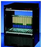
pation of 200 W per board. A 14 slot chassis can dissipate up to 2.8 kW.
