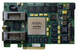
The A10 board family has flexible memory configurations, sophisticated clocking and timing options, QSFP28 cages that support 100 Gigabits per second (including 100 Gigabit Ethernet) optical transceivers, FPGA Mezzanine Card (FMC), and support for the network-enabled Altera SDK for OpenCL.
