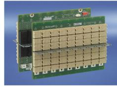
A maximum number of 9 slots are possible (one system slot and up to 8 peripheral slots). A robust coding pin in stainless steel allows use even in harsh environments.
